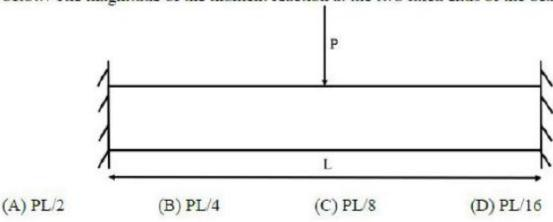
ANS: (C) Indeterminate beam, can be solved using Virtual work principle
